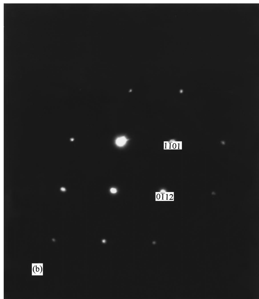
Figure 9 AlN formed in the higher Al steel after ageing at 850°C for 96 hours: (a) bright field image and (b) SAD pattern of AlN from zone axis of [01\bar{1}1] .
