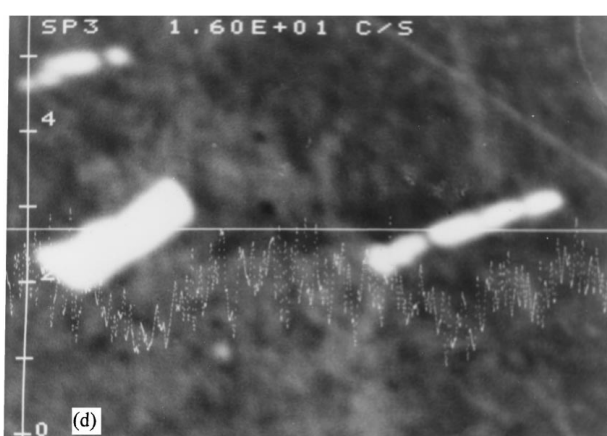
Figure 3 EPMA line scan analyses across precipitates in steel S1 after ageing at 850°C for 96 hours showing the larger precipitate is rich in Nb and Si and the smaller precipitate contains C and Nb. Sn was not detected in either type of precipitate: (a) Line scan of C, (b) Line scan of Nb, (c) Line scan of Si and (d) Line scan of Sn.
