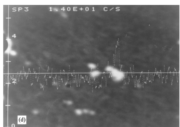
Figure 4 EPMA line scan analyses across precipitates in steel S2 after ageing at 850°C for 96 hours showing one type precipitate is rich in C and Nb and the other type of precipitate contains Nb, Si and Sn: (a) Line scan of C, (b) Line scan of Nb, (c) Line scan of Si and (d) Line scan of Sn.
